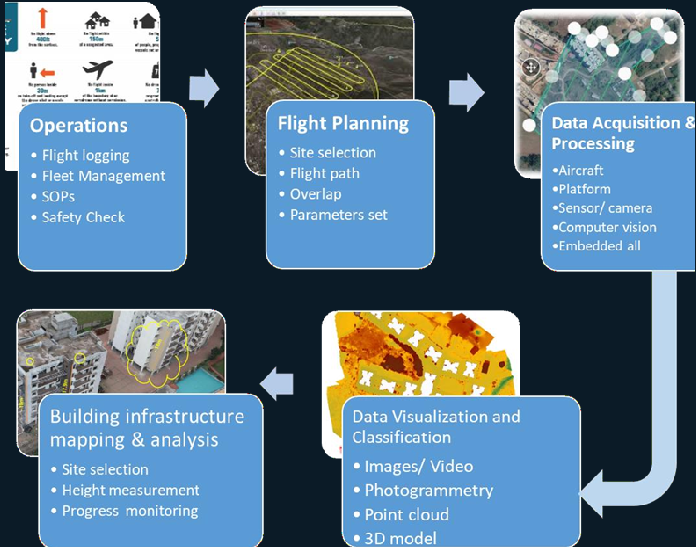
Simplified methodology process flow for feature extraction of building infrastructure mapping and monitoring using drone images
